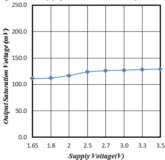
**Figure 5. Output Saturation Voltage vs. Supply Voltage**
