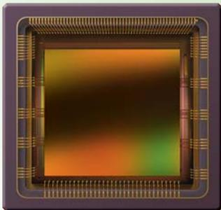
The CMV4000 is a high sensitivity, pipelined global shutter CMOS image sensor with 2048 x 2048 pixel resolution capable of HD format. Pipelining allows exposure during read out.
