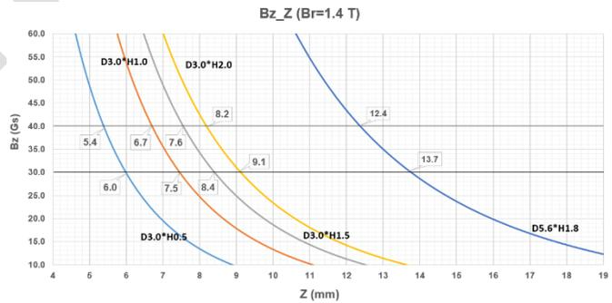
Figure 7: Field by magnet (different size and distance)
