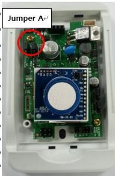
4 ~ 20mA is default (2 ~ 10VDC or 0 ~ 20mA or 0 ~ 10VDC is selectable with jumper setting change)
