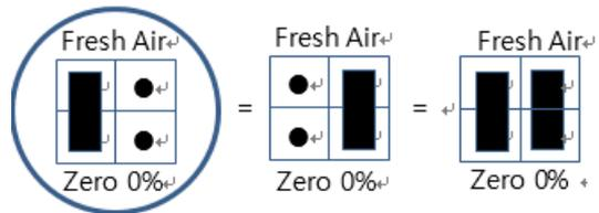
**Manual Zero Cal. mode-#2** is used to calibrate sensor with 0% O2 standard gas. Please make sure to locate O2-gas sensors on O2-gas-free area and move jumper setting from #1 to #2, which calibrate every minute. After calibration, return to previous set #1.
