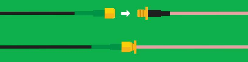
If you need to water proof a SMA connection, we highly recommend using a product like **Coax-Seal** to safely cover and prevent any water damage that may occur.
