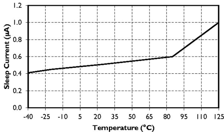
Figure 3. Sleep Current Variation over Temperature,  $V_{DD}$  at 3.3V
