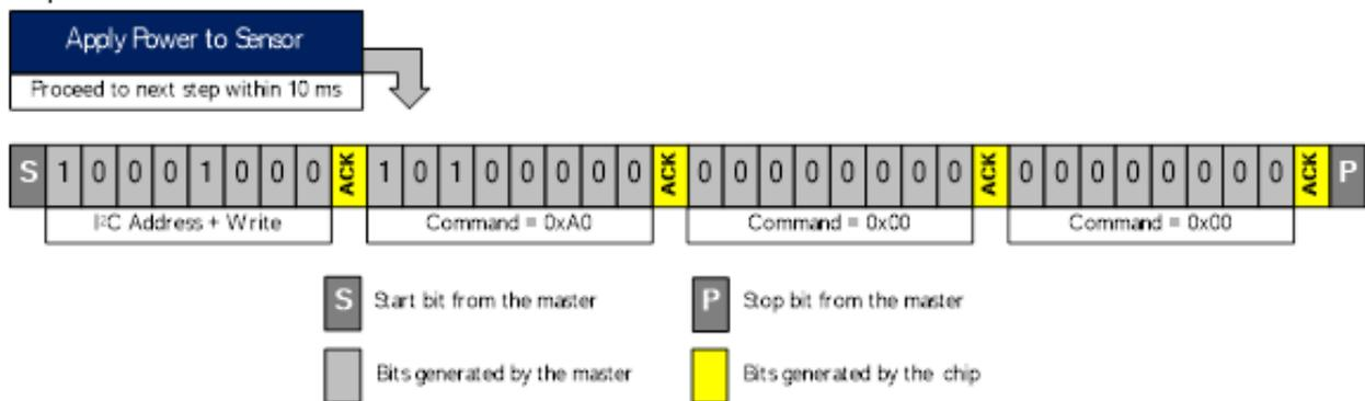
Figure 14. Sequence of Commands to Enter Programming Mode
