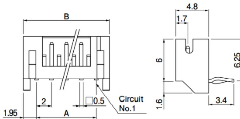
Figure 2. Pin Connector
