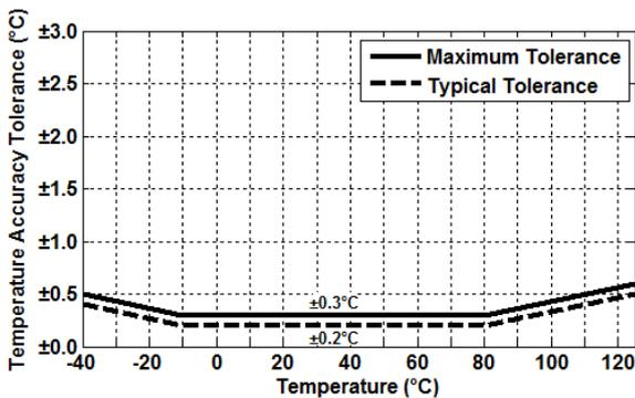
Figure 8. HS3101-MCx Temperature Sensor Accuracy Tolerance
