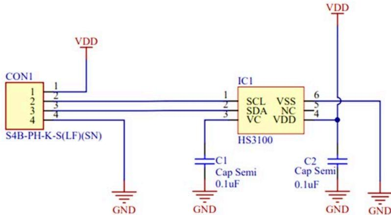
Figure 16. HS310x-MCx Application Circuit
