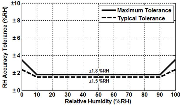
Figure 4. HS3101-MCx RH Accuracy Tolerance at 25°C
