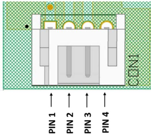
Figure 1. Pin Assignments
