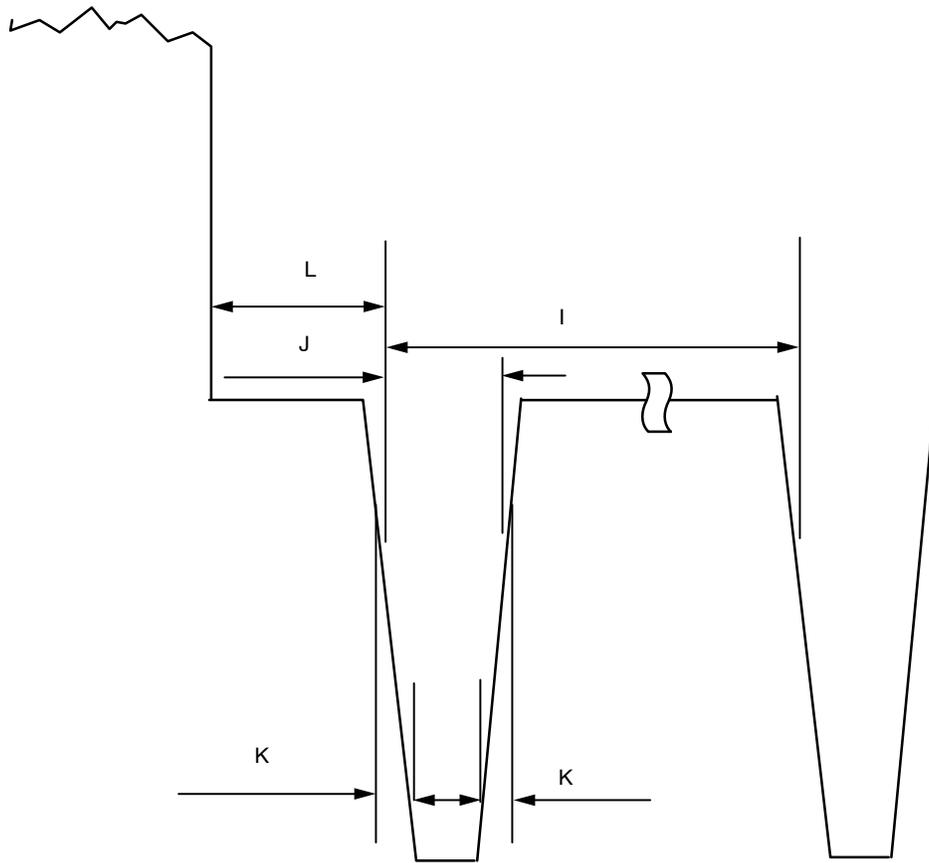
Figure 47. Equalizing Pulse
