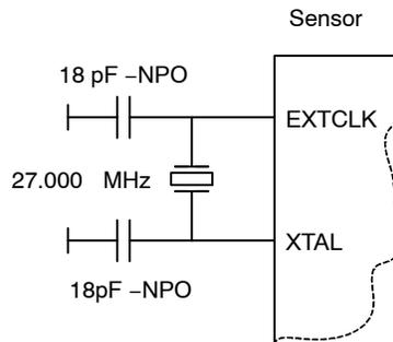
NOTE: Value of load capacitor is crystal dependent. Crystal with small load capacitor is recommended.
