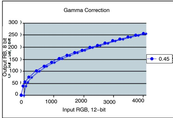
**Figure 11. Gamma Correction Curve**
