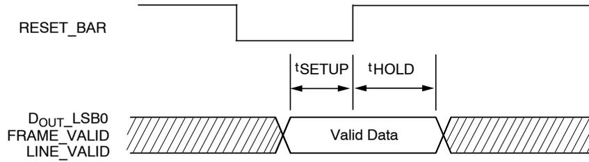
Figure 38. Configuration Timing
