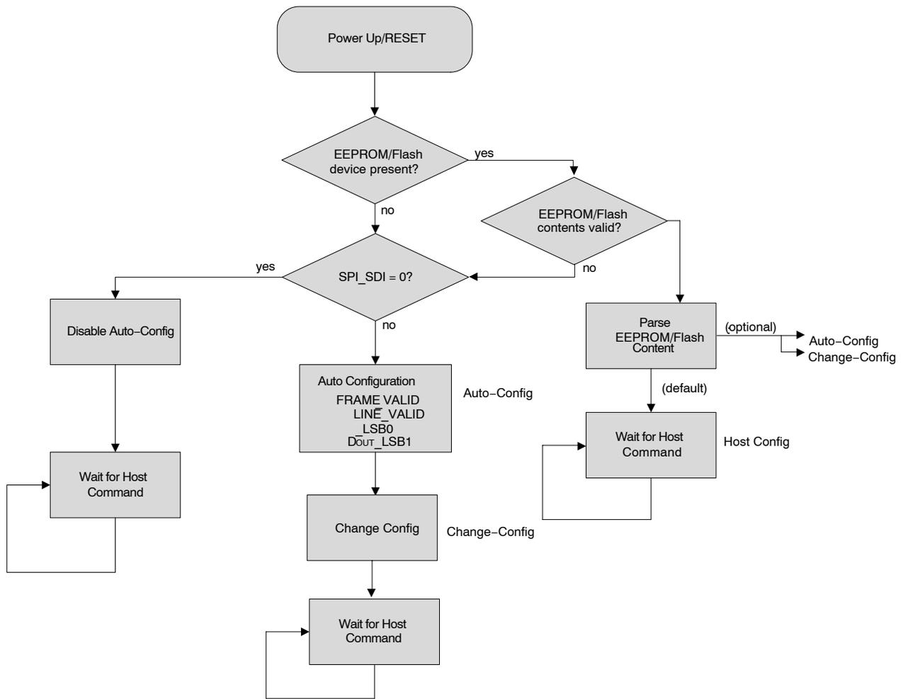
**Figure 14. Power-Up Sequence – Configuration Options Flow Chart**
