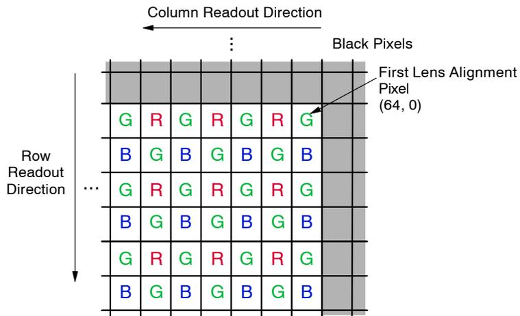
Figure 7. Pixel Color Pattern Detail (Top Right Corner)
