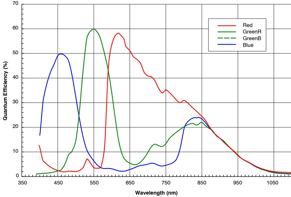
NOTE: The measurements were done on packaged parts with regular glass coating (that is, without Anti-Reflective Glass (ARC) coating).
