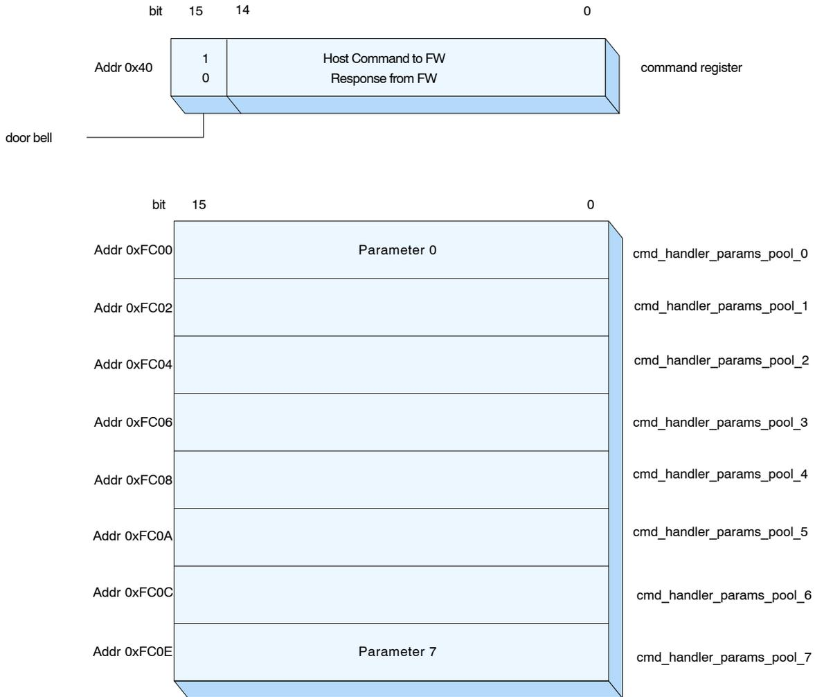
Figure 15. Interface Structure
