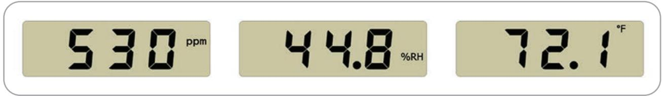
Display versions scroll between ppm CO<sub>2</sub>, %RH Humidity and °F Temperature when the option is selected.
