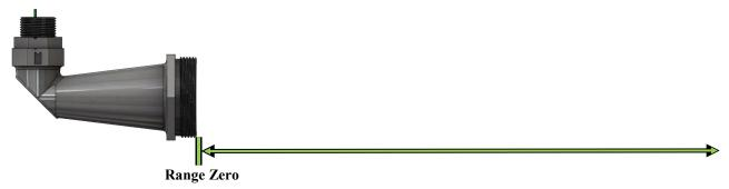
The range is measured from the front of the horn to the target.
