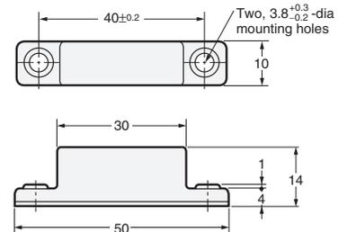
Note: The shape of the magnet is the same for Pre-wired Models and Terminal Block Models, but the magnet specifications are different.
