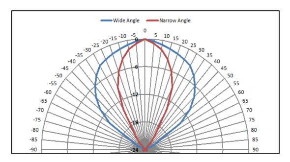
Note) Test Target : Φ75mm PVC Pipe at 100cm
