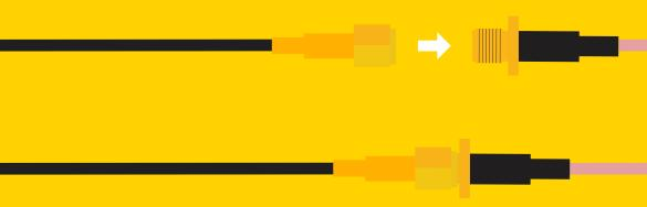
If you need to water proof a SMA connection, we highly recommend using a product like **Coax-Seal** to safely cover and prevent any water damage that may occur.
