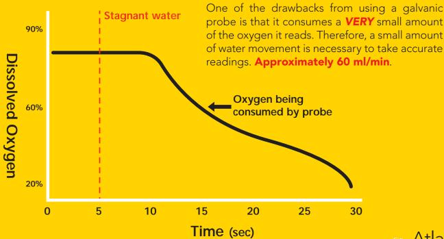
This galvanic dissolved oxygen probe is a passive device that generates a small voltage from 0mv – 60+ mv depending on the oxygen saturation of the PTFE sensing membrane. This voltage can easily be read by a multimeter or an analog to digital converter.
