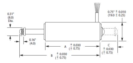
Dimensions are in inches (mm) (Refer to mechanical specifications for dimensions "A", "B" and "C")
