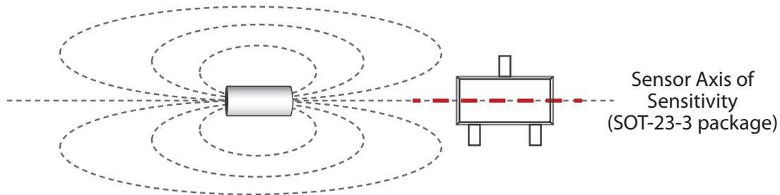
**Note:** The most straightforward way of aligning a magnet with a TMR sensor is by lining up the magnet's magnetization axis with the sensor's Axis of Sensitivity (as shown above). However, there are many other alignments and orientations that will also achieve proper operation. For any questions, or to learn more, please contact Coto Technology.
