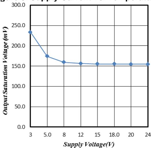
**Figure 5. Output Saturation Voltage vs. Supply Voltage**
