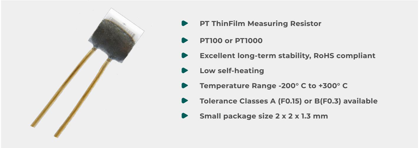
Variohm ERTD2 series ThinFilm Platinum Elements are durable and designed for applications where long term stability, interchangeability and accuracy over a large temperature range are important. Applications include automotive, white goods, HVACR, energy management, medical and industrial.
