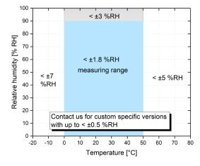
Fig. 1: Typical tolerance of the % RH measurement
