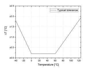
Fig. 2: Typical tolerance of the temperature measurement
