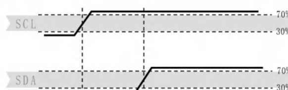
Figure 11. Stop transmission state (P)
