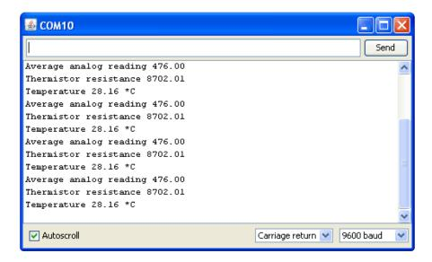
For better precision, we suggest reading the exact value of the 'series 10K' it should be nearly exactly 10K but if you can get a better reading that will reduce your error.
