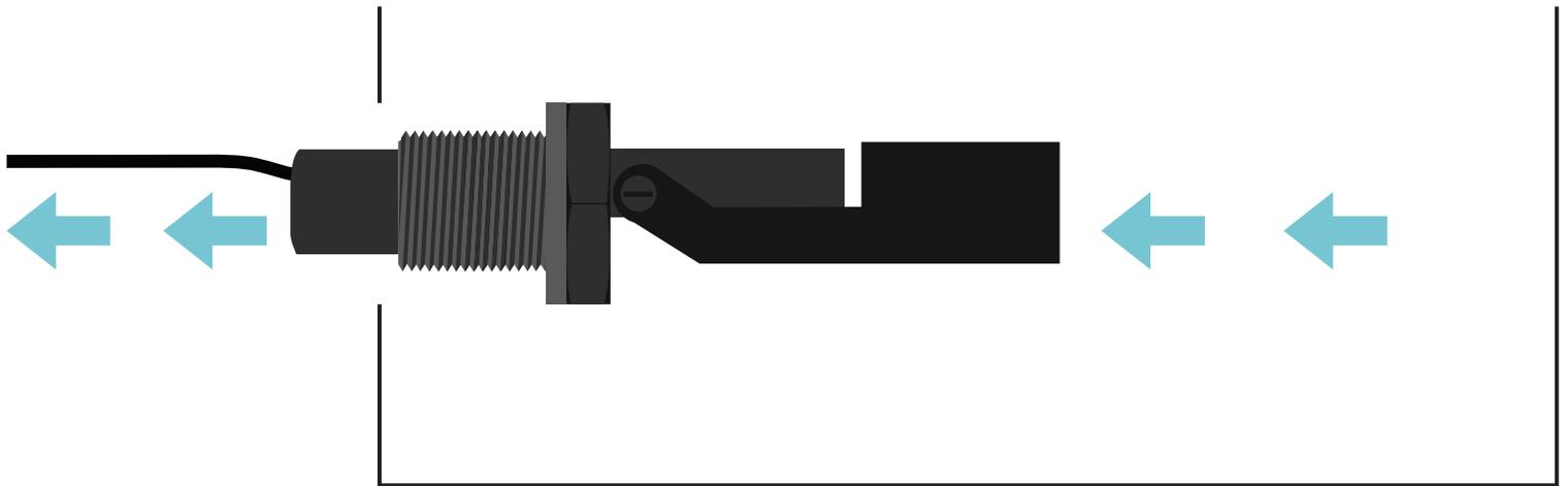
Now that the float switch is in place, re-attach and fully tighten the blukhead.
