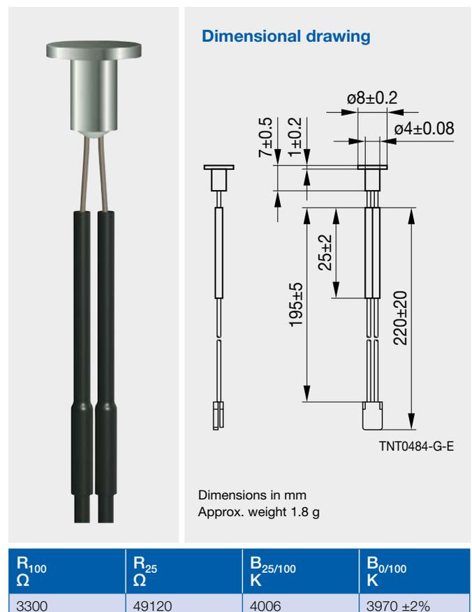
Figure 2: K560 surface temperature probe from TDK. Drawing and values taken from [3]
