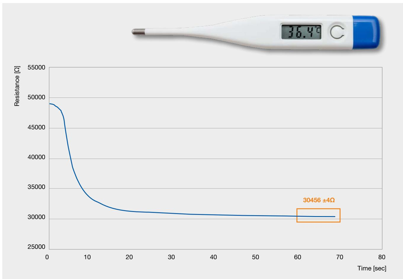
Figure 9: Example time plot for a calibration measurement
