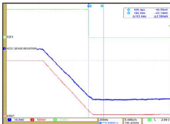
Figure 14: CT430 OCD enabled at -110\% of -50\text{ A}_{PK} and \overline{\text{FLT}} is Low
