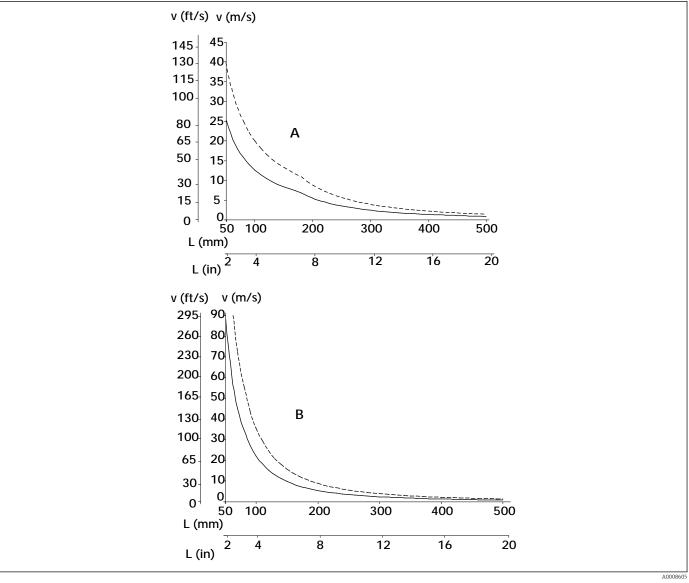
■ 8 Maximum flow velocity with thermowell diameter 9 mm (0.35 in)(-----) or 12 mm (0.47 in) (-----)
