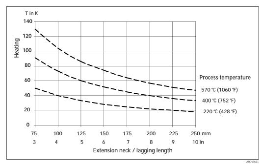
■ 11 Heating of the terminal head as a function of the process temperature. Temperature in terminal head = ambient temperature 20 °C (68 °F) +  $\Delta T$
