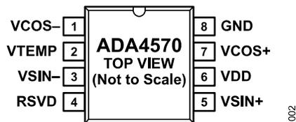
Figure 2. Pin Configuration
