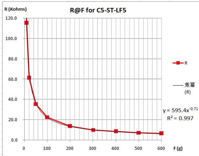
The following plot shows an near-linear curve which is  $1/R @F$ .
