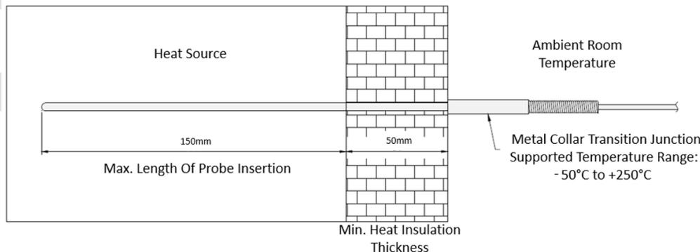
Figure 2: Probe and heat source
