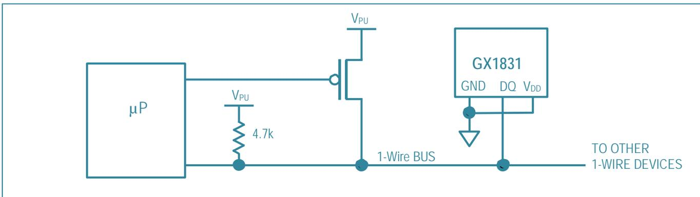
**Figure 5. Powering the GX1831 with an External Supply**
